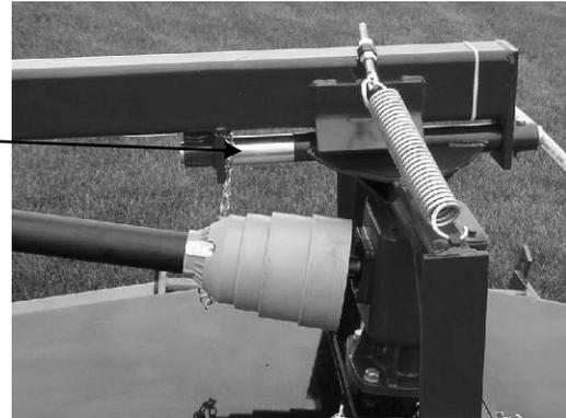
This spacer bushing can be mounted on either side of the wing deck swivel. Bushing shown mounted on the inside, positioning the wings out as far as possible. This will give maximum cutting width. Moving the bushing to the outside will increase the deck cutting overlap and reduce the overall cutting width. This will, however, reduce the width of the uncut strip when making turns. This position will be used when mowing while following a pivot track.
