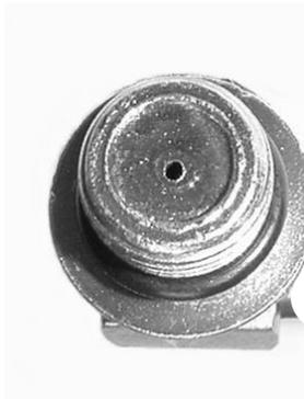
When reconnecting the quick disconnects to the tractor, be sure that both ends are clean. Dirt in the hydraulic system can block the orifice in the line throttle valve or even score the cylinder tubes.
